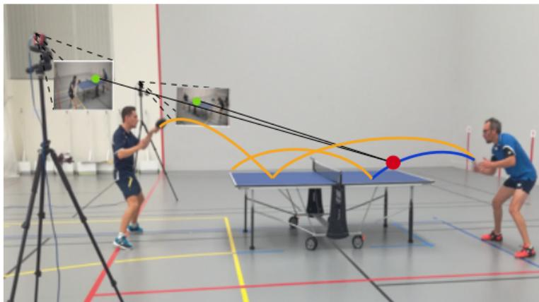
Figure – Frame from video sequences of Table-Tennis. Illustrate 3D reconstruction of ball using stereo-vision.
